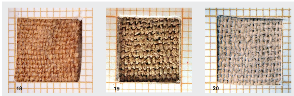
Figure 18. Example of medium density with thick yarns. 22 warp yarns x 14 weft yarns.
