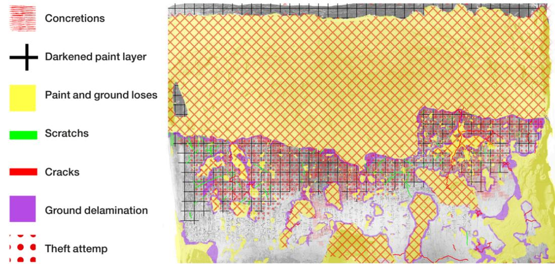
Figure 21. Damage map, with indication of the different types of alteration factors, corresponding to the east wall in the burial chamber of TT 61. I. Bermeja Gigorro.
