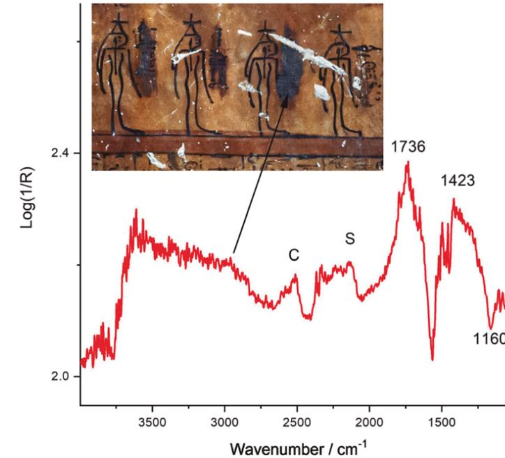
Figure 25. DRIFT spectra registered in a section of the Amduat on the east wall indicating the presence of gypsum (S), calcite (C), and organic binders (glue and oil/wax). S. Sánchez-Cortés, S. Martínez Ramírez, and D. Méndez-Rodríguez.
